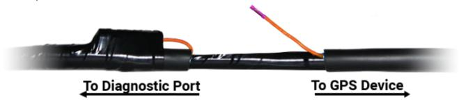
Remove 1 in. of sheathing from the inline fuse holder and butt connect the fuse holder to wire leading to the GPS device connection before taping off and cable tying connection.
