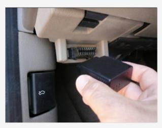
b. Secure the device to the OBD-II Port with a zip tie and ensure connection secure.
