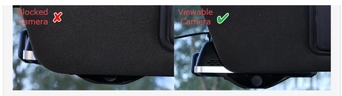
• Type 2: Rear View Mirror (Sensor Housing/Large Trim); Right side of housing/trim with bracket bottom the same level as housing.
