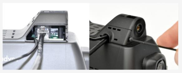
3. Cable tie the antenna cable to the rear-view mirror wires, route the antenna along the headliner and down the a-pillar securing with cable ties ever foot.
