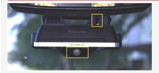
1. Place the device into the mounting bracket and lightly screw in the mounting bolts. Do not fully tighten down screws as the camera may need to be adjusted in Step 3.
