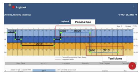
The distance traveled while in PU and/or YM status is included in the daily odometer shown in the Logbook and the Print/Display option of the Portal.
