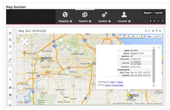
The Map Dashlet shows a 2D map with current locations of a selected vehicle group. Edit options allow you to filter by vehicle status (running, stopped, stopped for a set time period). You can also adjust vehicle/driver labels, add landmarks to the map, adjust map height and zoom options, and more. On the map control, toggle between Clusters, Traffic, Service Reminders, Points of Interest, Map View, Satellite View, or Street View.
